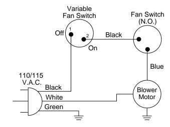
Figure 63 - Blower Wiring Diagram for Thermostat-Controlled Models
